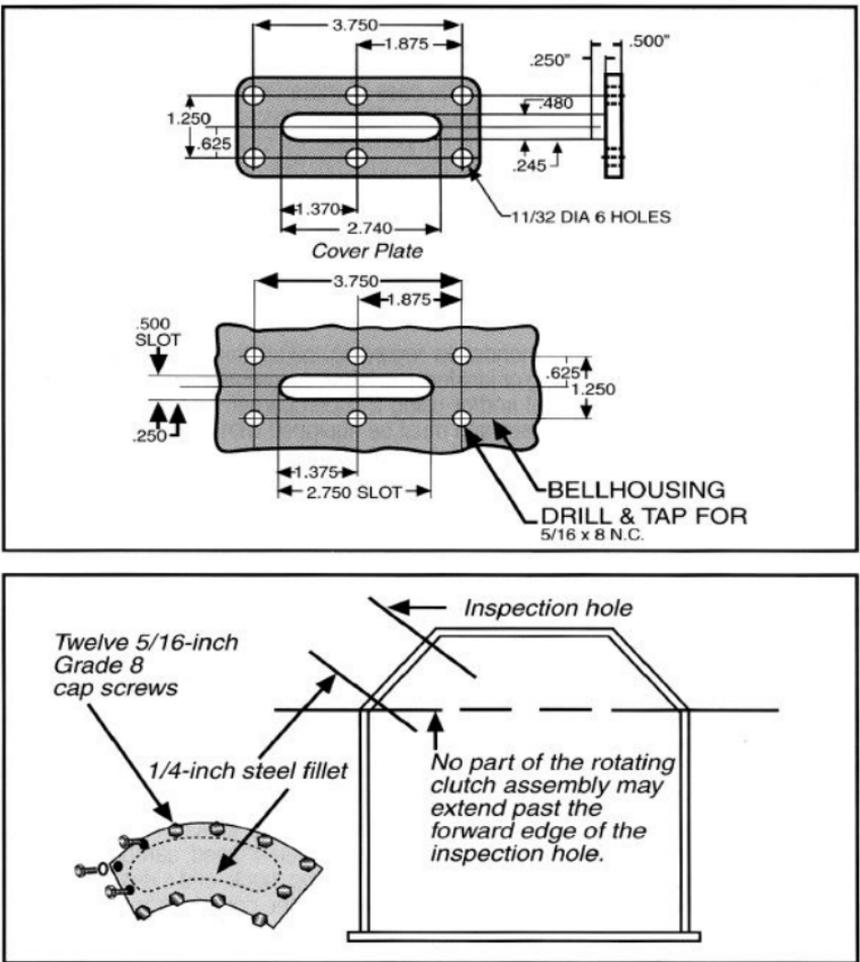
Figure 3 and 4: Bellhousing inspection hole cover
