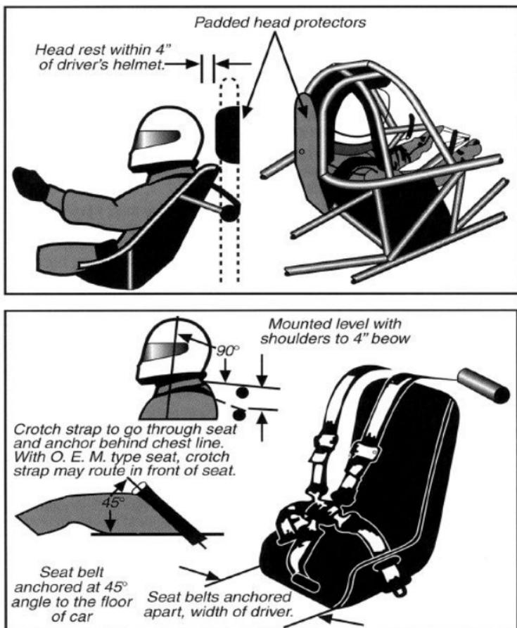
**Figure 12 and 13: Head protectors and harness mounting**
