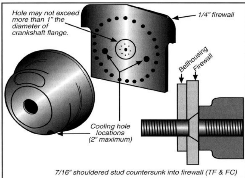
**Figure 5: Motor plate**
