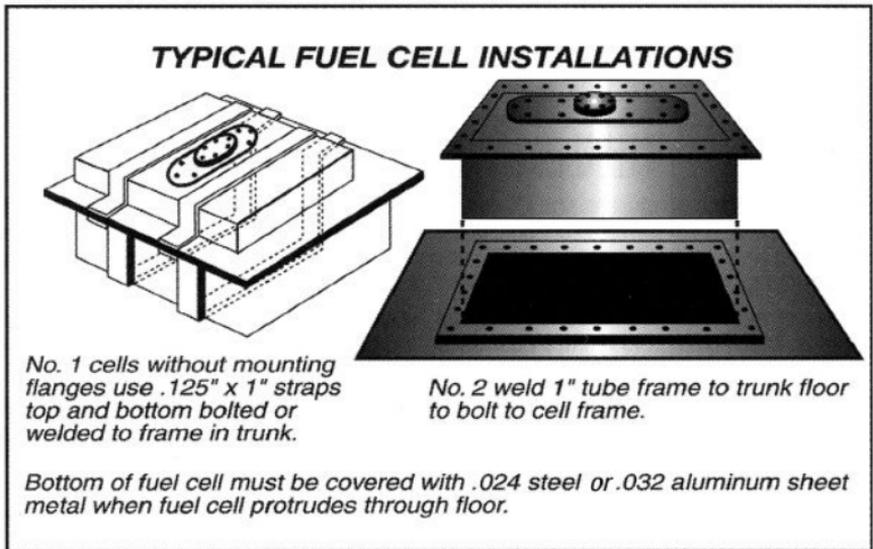
**Figure 6: Fuel cell installation**
