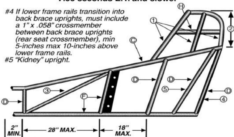
Figure 9: Rear-Engine Dragster roll cage
